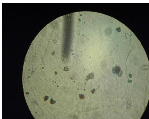
Fig. 4. Micrograph of dispersed residue of ras from low-paraffin oils
